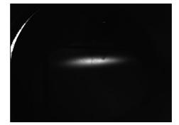
Fig. 2. A beam of  ${}^{56}$ Fe ${}^{14+}$  ions on the phosphor screen at the end section of the Booster–Nuclotron transport channel
