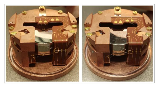
Fig. 2. Photos of a planar (left) and an FID (right) detector prototype made by EDELWEISS/Ricochet for Dark Matter search and precision study of  $CE\nu NS$
