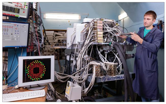
The Flerov Laboratory of Nuclear Reactions. The SFiNX detector system of the SHELS separator for studies of the properties of the spontaneously splitting short-lived nuclei obtained in reactions with heavy ions
