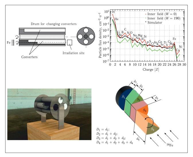
Fig. 8. An illustration of the concept of a new GCR simulator: a schematic of a drum for changing converters, a graph of the produced integral value of the particle fluence at the irradiation site, and a 3D schematic of a separate converter
