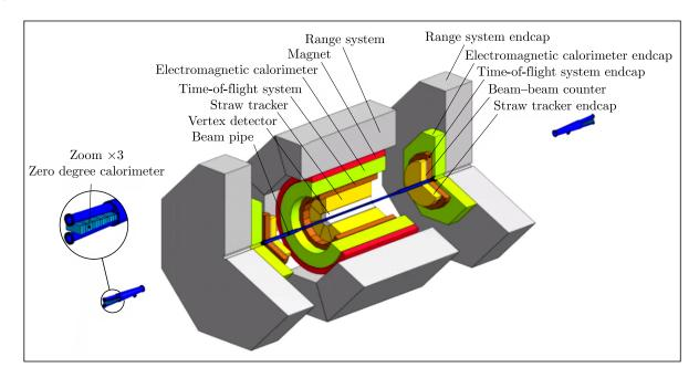
Fig. 6. Upgraded configuration of the SPD detector
