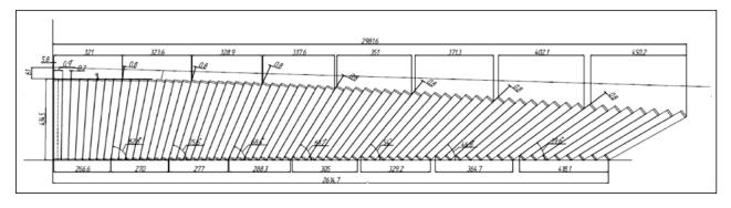
Fig. 3. Layout of the towers in the half-sector of the electromagnetic calorimeter with a projective geometry
