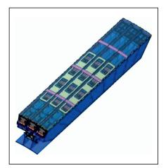
Fig. 4. ECal basket with electronics
