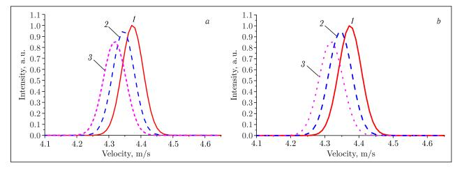
Fig. 4. a) Velocity spectra of UCN that passed over an accelerating potential barrier as a function of the barrier height: I - initial spectrum; 2 - U = 50 neV; 3 - U = 75 neV; b) velocity spectra of UCN that passed over an accelerating potential well: I - initial spectrum; 2 - well depth 50 neV; 3 - well depth 75 neV
