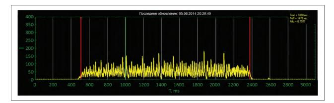
Fig. 2. Intensity time dependence of the extracted  ${}^{40}Ar^{16+}$  beam. Energy is 1.2 GeV/u, total ion number is  $1.5 \cdot 10^5$ , the spill duration is 2 s
