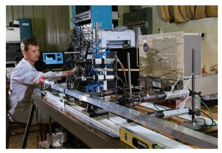
The Dzhelepov Laboratory of Nuclear Problems. An experimental test stand for studies of the properties of plastic scintillation strips
