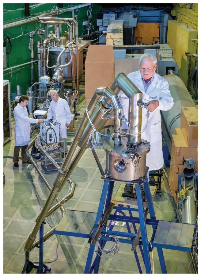
The Frank Laboratory of Neutron Physics. The test stand of the cryogenic neutron moderator of the IBR-2 reactor
