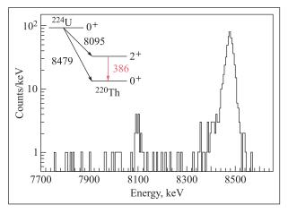
Fig. 3. Spectrum of  $\alpha$  decay of <sup>220</sup>Th
