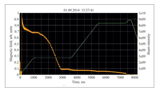
Fig. 1. The magnetic field cycle and beam intensity in the double user mode. At the first flat-top, the beam intensity decreases due to interaction with the internal target, at the second flat-top, the slow extraction is provided. At the both plateaus, RF is off
