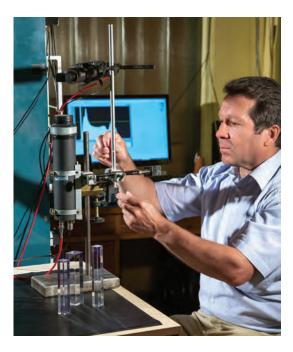
The Dzhelepov Laboratory of Nuclear Problems. An experimental test stand for studies of the properties of scintillation crystals
