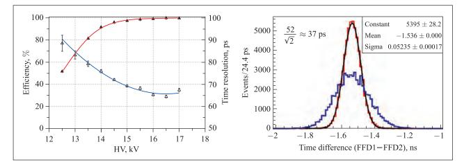
Fig. 3. Time resolution and efficiency of the MRPC strip for the time-of-flight system (left); time distribution between two identical prototypes of FFD (right)
