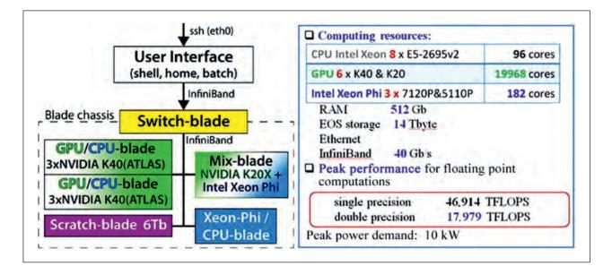
Fig. 3. The structure of the heterogeneous computing cluster HybriLIT (left). The main parameters of the computational elements of the cluster and its efficiency (right)
