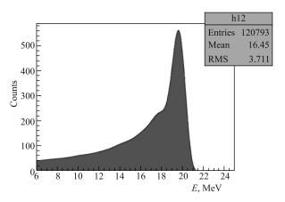
Fig. 6. The simulation of 19.8 MeV  $\gamma$  energy spectrum inside BGO crystal
