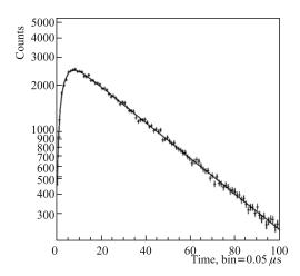
Fig. 8. The  $\gamma$  time spectrum, simulated according to expression (9) with the initial values  $\lambda_{pt\mu} = 6.5 \ \mu s^{-1}$  and  $\lambda_{pt}^f = 0.067 \ \mu s^{-1}$ . Line reflects the fit result
