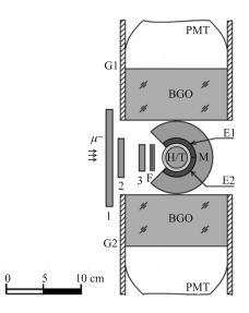
Fig. 4. The proposed installation: 1–3 — muon telescope plastic counters; BGO — scintillation crystals; E1, E2 — electron plastic counters; F — copper degrader; G1, G2 — gamma detectors; H/T — target; M — muon plastic counter; PMT — photomultiplier
