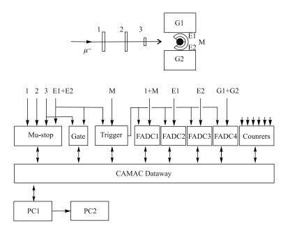
Fig. 7. Block diagram of the electronics
