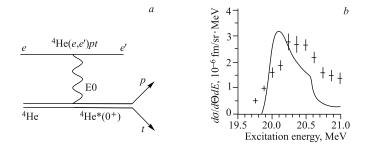
Fig. 1. Diagram for  ${}^{4}\text{He}(e, e')pt$  process (a) and the appropriate cross section (b)
