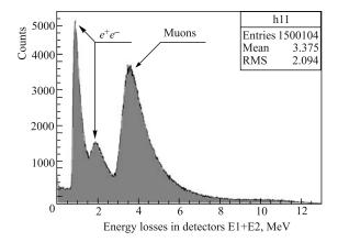
Fig. 5. The simulated sum ( $\mu$  and  $e^+e^-$ ) energy spectrum in detectors E1 + E2
