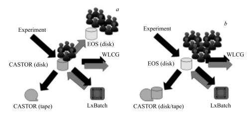
Fig. 1. The simplified schemas for the data handling at the CERN Tier-0. The black arrows represent the raw data and the grey ones are the data generated by the reconstruction. a) The schema used by ALICE and LHCb. The CASTOR disk front-end is directly used for reconstruction, while the analysis uses EOS disk. b) In the ATLAS and CMS scheme, EOS handles all the user activities, while the CASTOR disk acts as cache for the tape system
