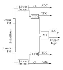
Fig. 3. Scheme of the electronic channel of an FSH counter
