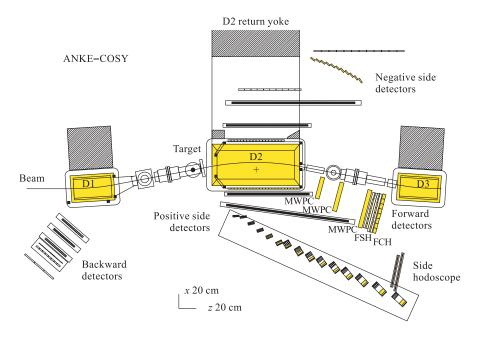
Fig. 1. Scheme of the ANKE setup
