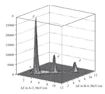
Fig. 4. Energy loss distribution in two matching counters of the scintillation hodoscope measured at a beam energy of 0.5 GeV with a hydrogen target
