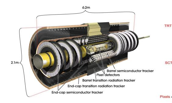
Silicon pixels (**Pixel**): 0.8 10<sup>8</sup> channels Silicon strips (SCT) : 6 10<sup>6</sup> channels Transition Radiation Tracker (TRT) : straw tubes (Xe), 4 10<sup>5</sup> channels  $e/\pi$  separation
