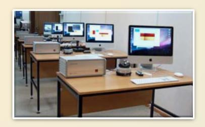
3 scanning probe microscopes
